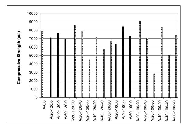
Not statistically different mixtures in ninety-day compressive strength between GR 100 GGBFS and GR 120 GGBFS were: A/20/0, A/40/0, A/60/0, A/20/20, A/20/40, and A/40/40. The A/40/20 and A/60/20 mixtures were decreased by 11% when made with GR 120 GGBFS. The A/20/60 mixture had a 15% decrease in ninety-day compressive strength when made with GR 100 GGBFS. The 90 day compressive strength trends observed were as follows from the data and Chart 4.33:
