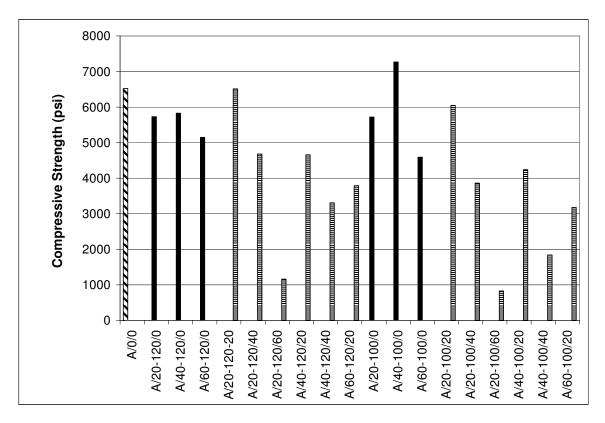
The mixtures that had not statistically different twenty-eight day strengths whether they were made with GR 100 or GR 120 GGBFS were A/20/0, A/20/20, A/20/60, and A/40/40. Four of the remaining five mixtures had greater twenty-eight day compressive strength when made with GR 100 GGBFS. These mixtures were A/40/0, A/60/0, A/20/20, A/40/20, and A/60/20. The trends in twenty-eight day compressive strength data and Chart4.32 were observed to be as follows:
