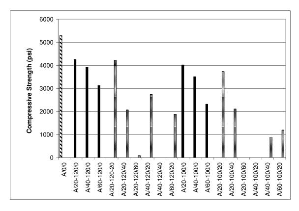
At seven days of age, the A/20/0, A/20/60, A/40/40, and A/60/20 mixtures had not statistically different compressive strengths between the GR 100 and GR 120 GGBFS mixtures. The A/60/0, A/20/20, A/20/40, and A/40/20 mixtures saw a 11%, 7%, 2%, and 9% decrease in compressive strength with GR 100 GGBFS. The A/40/0 mixture had a 20% decrease in strength when made with GR 120 GGBFS. The 7day compressive strength trends were observed to be as follows from the data and Chart 4.31:
