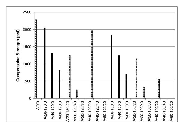
At three days of age, mixtures that had not statistically different compressive strengths were A/20/0, A/20/40, A/20/60, A/40/40, and A/60/20. The A/40/0, A/60/0, and A/20/20 mixtures had an average of 14% less three-day compressive strength
