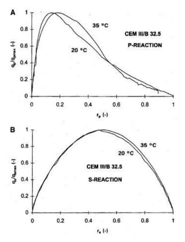
The reaction curves show that portland cement mixtures gain heat more rapidly than GGBFS. The heat gain curves also show slag cement heat gain begins later than the portland cement, explaining the slower heat of hydration and the increase in set times for mixtures containing GGBFS (Schutter, 1999).
