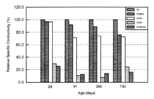
The conductivity is attributed to the pore structure and pore solution characteristics while the transport of chloride ions in the ponding and pressure tests is attributed to the pore structure. The recommendations from the research conclude that the passed
