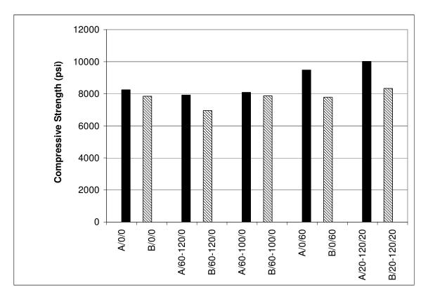
The cement study suggested that the two sources of cement did not create the same compressive strengths with the same replacement mixtures. They, however, had similar trends in mixtures with similar replacements of cement. The replacements of
